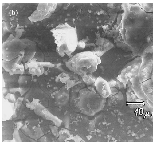
Fig. 6. SEM micrograph of magnesium deposit on nickel substrate. (a) Q = 1.35 \text{ C cm}^{-2} ; (b) Q = 7.2 \text{ C cm}^{-2} .
